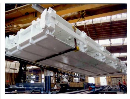
The cage head is equipped with a suspension board to enable installation of the necessary amount of upper brackets. Under the cage foot there are supports that enable installation of the required amount of balancing rope suspensions. Under the cage head and cage foot, there are foots in order to enable container chocking, or its placement on the foldaway supports.
